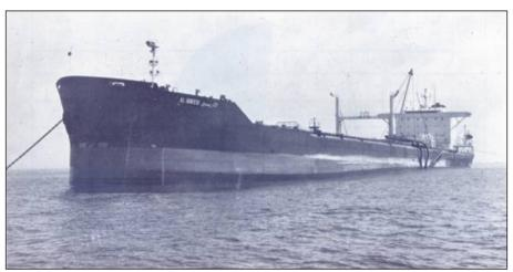
figure -4: Tanker AL IDRISSI (1976–1986); 51,546 tx gross tonnage, length 257 m; built in Italy (Ancona) in 1976; docked at the sea-line (Mohammedia) after the maiden trip in 1976; photo: Cherfaoui Najib.
