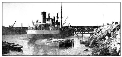
**figure 7:** First tanker under Moroccan flag; purchased brand-new, the ship FEDHALA owned by the « Compagnie Marocaine des Transports Maritimes », during unloading operation (1926) at the port of Fédala (Mohammedia); built at the Chantiers Navals Français (Blainville); length 49 m, gross tonnage 522 tx; 600 hp engine; (photo: Helderline Shell Tanker).
